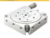
7R129 is Vacuum Compatible Precision Rotary Stage with a micrometer screw. Fine motion range is 15° with resolution of 1 arcmin. The platform has mounting holes M6, M4. Precision rotary stage has an aperture M30x1 with clear aperture of 25 mm. Precision rotary stage can be fastened horizontally and vertically using M6 screws.
