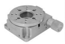
The main advantage of this precise rotation stage is that it has very compact dimensions and low-profile together with the great aperture in the middle. This rotation stage has two modifications with different apertures: M27x1 or 30 mm. 7R150V doesn't need additional adapter plate to be mounted on any surface as it has 3 M6 holes on bottom.
