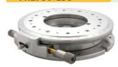
7R170V-190 is used to rotate manually large optical and other components through continuous 360° with accuracy of 1°, and finely to adjust them within 10° by a micrometer, with accuracy of 0.5arcmin. The stage has 88.9 mm clear aperture. The platform of the stage has a pattern of M6 and M4 mounting holes for components.
