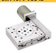
8MT167V-VSS42 is motorized translation stage for vacuum motion control application where load capacity and value of stage is combined. Fabricated using high temperature stability age hardened aluminum alloy. Precise, low backlash lead screw transmission guarantees stable and highly repeatable motion in vertical and horizontal orientation.
