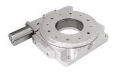
8MR190V-90-VSS43 is motorized vacuum compatible rotation stage for highly loaded applications motion control application. Fabricated using high temperature stability age hardened aluminum alloy. Precise, low backlash worm gear guarantees stable and highly repeatable motion in vertical and horizontal orientation
