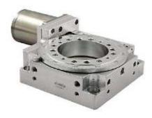
8MR190V-2-VSS42 motorized rotation stage with 50.4 mm aperture most efficient solution for vacuum compatible motion control application where load capacity and value of stage is combined. Fabricated using high temperature stability age hardened aluminum alloy. Precise, low backlash calibrated worm gear guarantees stable and highly repeatable motion in vertical and horizontal orientation.
