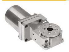
8MR174V-11 motorized rotation stage is compact solution for vacuum compatible motion control. Fabricated using high temperature stability, age hardened aluminum alloy. Precise, low backlash calibrated worm gear guarantees stable and highly repeatable motion in vertical and horizontal orientation. Special ultrasound cleaning and lubricants results low outgassing in extremely clean environments.
