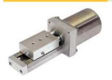
8MT173V is compact motorized translation stage for vacuum compatible motion control. Fabricated using high temperature stability, age hardened aluminum alloy. Precise, low backlash lead screw transmission guarantees stable and highly repeatable motion in vertical and horizontal orientation.
