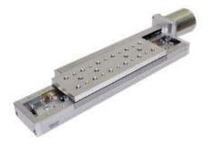
8MT167V-VSS42 is long travel range motorized translation stage for vacuum motion control. Fabricated using high temperature stability age hardened aluminum alloy. Precise, low backlash lead screw transmission guarantees stable and highly repeatable motion in vertical and horizontal orientation.
