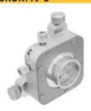
Five-Axis Optical Mounts consist of side Specifications regulation two-axis kinematic mirror mount with two screws, two-axis translation stage with 2mm travel range driven by two screws and zoom which provides 10mm travel range. Five-Axis Optical Mounts hold 1-inch optics. In addition, the adapters may be purchased to mount optics of different diameters. The mounts have M6 holes on the bottom to accommodate different mounting systems directly or through thread adapters.
