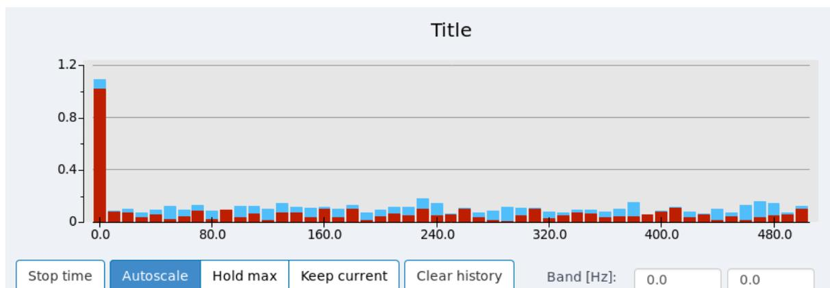
Figure 7.15 The spectrum graph on the “Dashboard” page (red columns - current spectrum, blue columns - maximal amplitudes)
