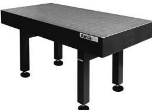
Optical Table Support 1TS with Honeycomb Table Tops 1HT
