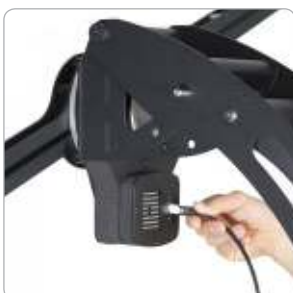
The 2-axis goniometer gives you a full 3D light distribution
