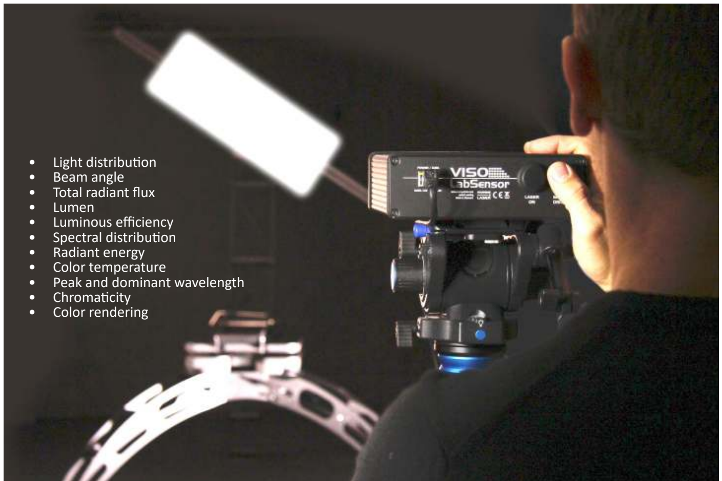
The 2-axis goniometer gives you a full 3D light distribution
