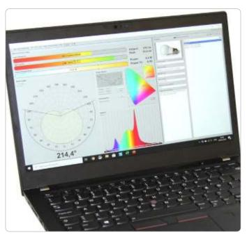
The Viso Light Inspector software is included. The software controls the fully automatic measuring process, all settings and outputs and your measurement library.
