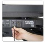
The main board easily slides out allowing a quick update
