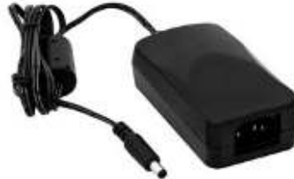
Power supply PSC30U-120V 12 V; 2.5 A 98.5 × 55 × 31.5 mm 250 g connector “2.1/5.5”
