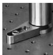
3UTC clamp the rod exactly at the middle (page 3-4)
