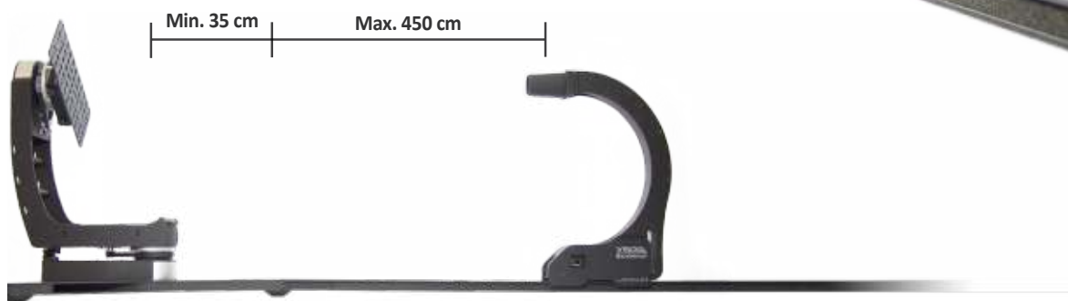
The universal light source bracket easily clicks onto the goniometer
