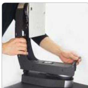
Before measurement, simply slide, align and lock the light source to the center
