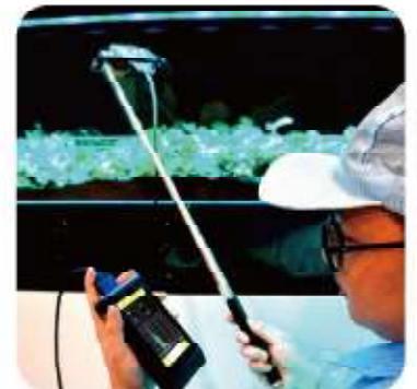
Sensor head can be used with a selfie stick and camera tripod. Users can easily measure far reaching ranges and adjust the measurement point horizontally.
